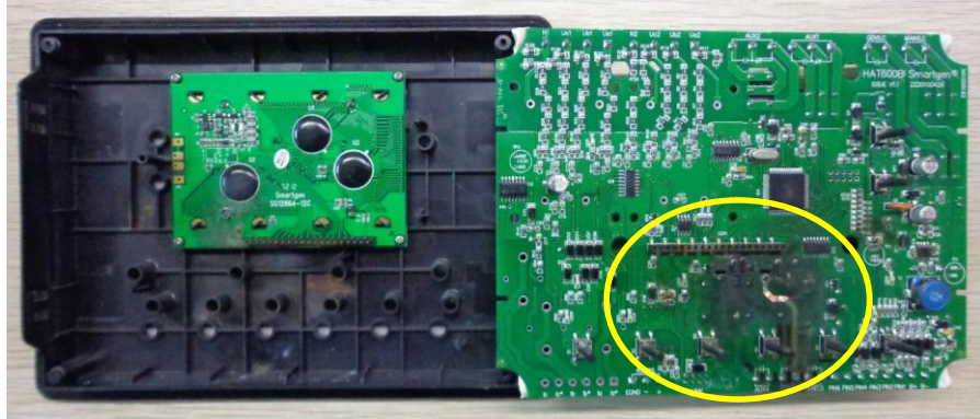
Figure 2 – An example of an ATS circuit board that burned from electrical surge.
